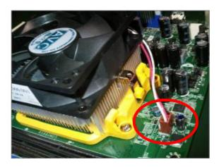
7.8 Release two side buckles and rotate latch of CPU Cooler then remove it
